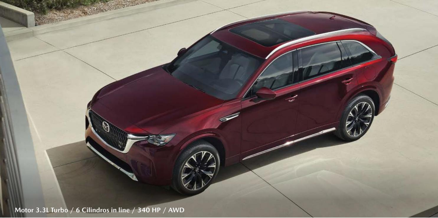
Motor 3.3L Turbo / 6 Cilindros in line / 340 HP / AWD
